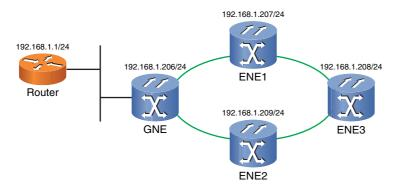
Successful ping responses to both ENEs from the router result in the ARP cache, as shown in Listing 3-1. The GNE's MAC address is mapped to all three IP addresses, an indication that GNE is performing PAS for the three ENEs. In other words, all three ENEs are PAS clients.
