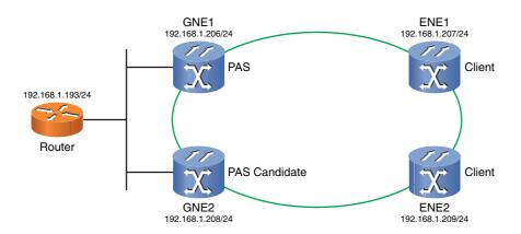
If both GNEs lose visibility over DCC to each other, either by dual-fiber breaks or disabling of OSPF on links connecting the two GNEs, a special case is formed where, although both GNEs are still on the same LAN segment, they do not share the same OSPF database. As a result, the two GNEs do not see each other and the respective ENEs as peers. A new PAS-client relationship is formed.
