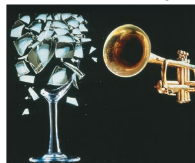
FIGURE 14–25 A goblet breaks as it vibrates in resonance to a trumpet call.
