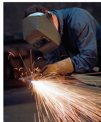
A mixture of acetylene and oxygen undergoes combustion during the welding of metals.
