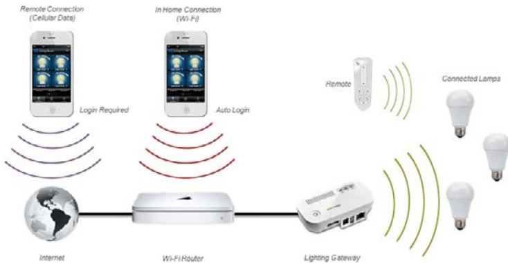
Figure 5.2 The Connected by TCP smart lighting system.
