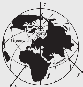
Figure 3.4 Rectangular Coordinate System for the Earth.
