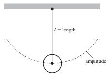
(*Note:* The amplitude of a pendulum has no effect on its period. This is what makes pendulums such good time-keepers. Because they invariably lose energy due to friction, their amplitude decreases but their period remains constant.)
