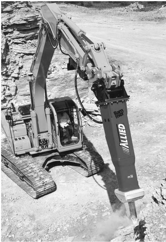
FIGURE 14. Hydraulic demolition hammer. (Courtesy of Allied Construction Products, Inc.)
