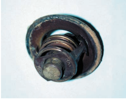
FIGURE 6 A thermostat stuck in the open position caused the engine to operate too cold. If a thermostat is stuck closed, this can cause the engine to overheat.
