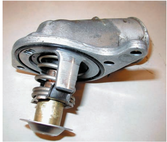
FIGURE 10 Some thermostats are an integral part of the housing. This thermostat and radiator hose housing is serviced as an assembly. Some thermostats snap into the engine radiator fill tube underneath the pressure cap.
