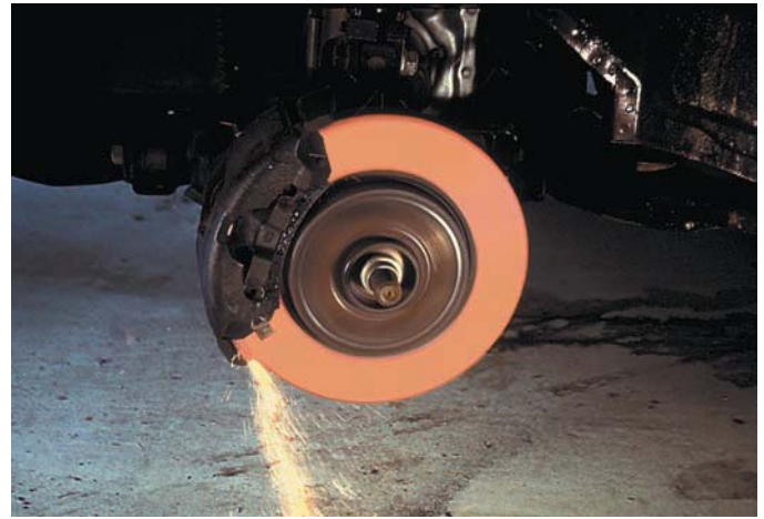
FIGURE 3 Disc brakes can absorb and dissipate a great deal of heat. During this demonstration, the brakes were gently applied as the engine drove the front wheels until the rotor became cherry red. During normal braking, the rotor temperature can exceed 350°F (180°C), and about 1,500°F (800°C) on a race vehicle.
