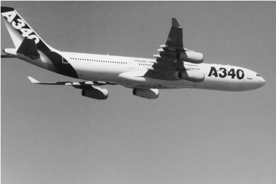
Fig. 4.17 Wing-tip winglets on the Airbus A340 reduce drag
