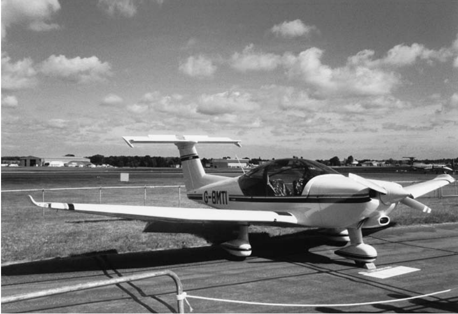
Fig. 4.14 Bent tips on the Aerospatiale Robin
