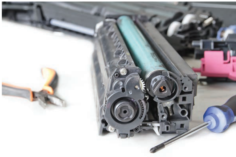
FIGURE 9.11 Inside a laser printer cartridge
