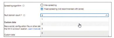
FIGURE 2-18 Set the fault domain count.
