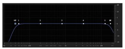
A Highpass response progressively reduces response below a certain frequency (called the *cutoff frequency*); the lower the frequency is below the cutoff, the greater the reduction. A Highpass filter is helpful for removing subsonic (very low-frequency) energy.
