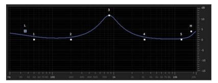
Reload the Default preset so the EQ has no effect. There are two additional stages, Highpass and Lowpass, which you enable by clicking the HP and LP buttons, respectively. Click those buttons now.
