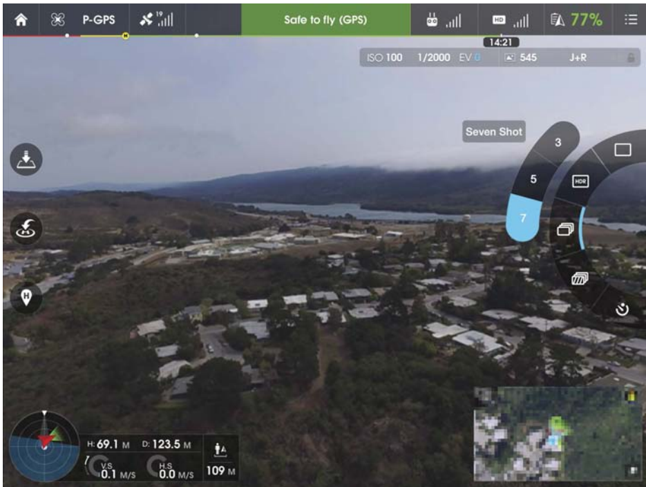
FIGURE 3.7 Burst mode controls in the DJI GO app for Phantom 3 and Inspire 1, with Seven Shot selected
